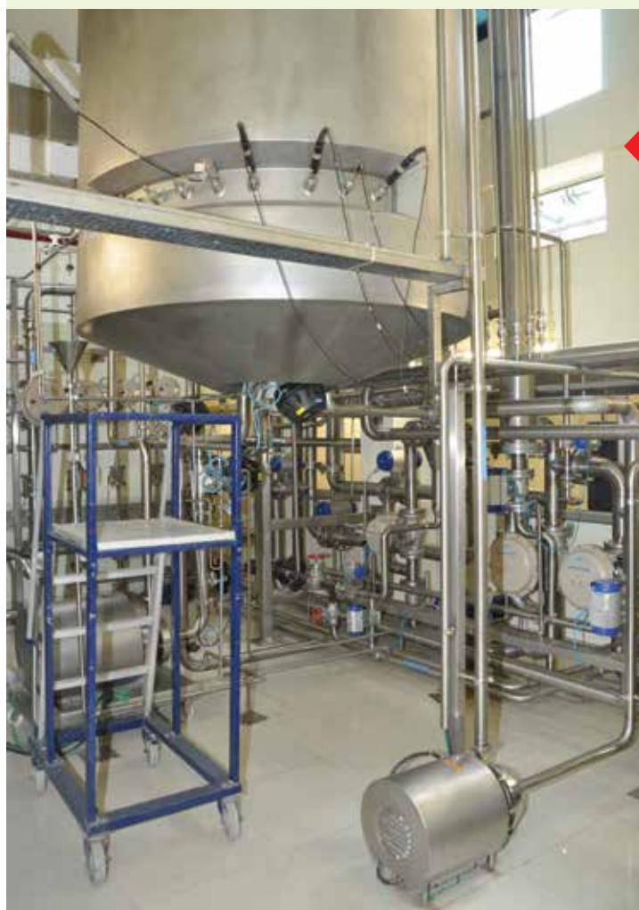
○ Bottom view of 13,000 L bioreactor used for large scale production of KT-Oilzapper
