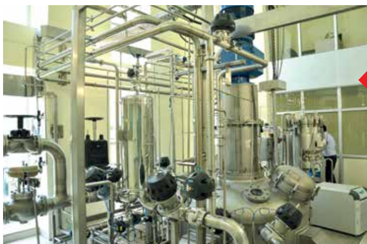
○ Top view of 13,000 L bioreactor used for large scale production of KT-Oilzapper
