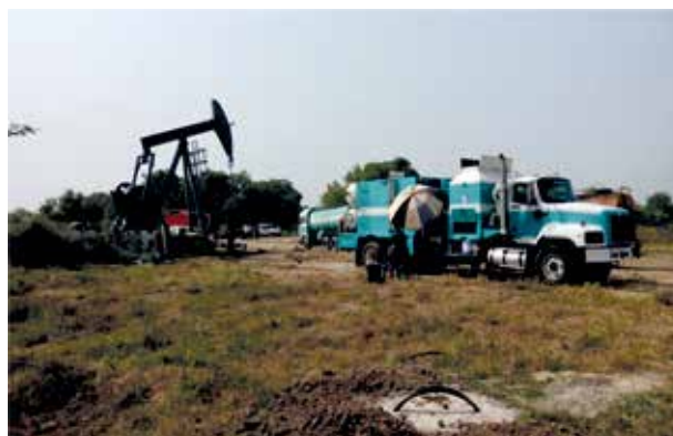
○ Field-scale injection of 'B-90' microbial culture into heavy oil well reserve of ONGC
