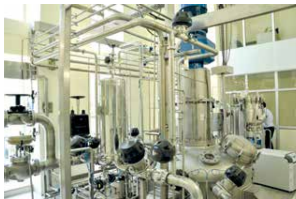
○ Large-scale (200,000 litre) preparation of heavy oil degrading themophilic 'B-90' microbial culture in anaerobic condition, at TERI's state-of-art Fermentation Technology Research Centre
